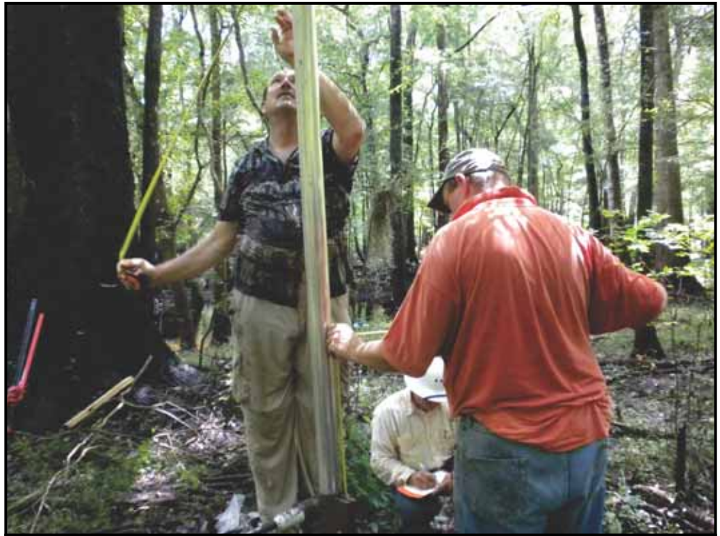
Norden site coring operation left to right, Glen Doran measuring up, Jack Rink taking notes, and Charles Fredrick measuring down. Coring device is Jack Rink's Vibra-Core donated to ARI.
